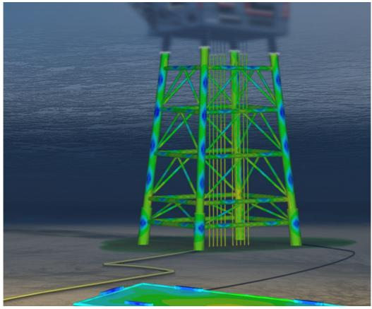
Imenco provides complete cathodic protection systems Imenco has produced ROV installable Retrofit Anode Systems since 1999, which have proved to be very effective and installation friendly. The smart solution cater for compact design, enabling great flexibility in anode attachments.
